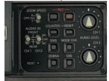
Sub-panel buttons, switches and Audio level controls behind the LCD panel
